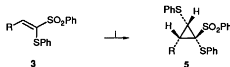
Scheme 2 Reagents and conditions: i, Li-4, THF, -78 to 0^\circ\text{C} or room temp.
